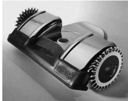
Fig.3.9 Cye, a commercial two-wheel differential-drive robot
