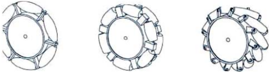
Fig.3.4 Omnidirectional Wheels, form left to right: Universal, Double Universal, Swedish 45°
